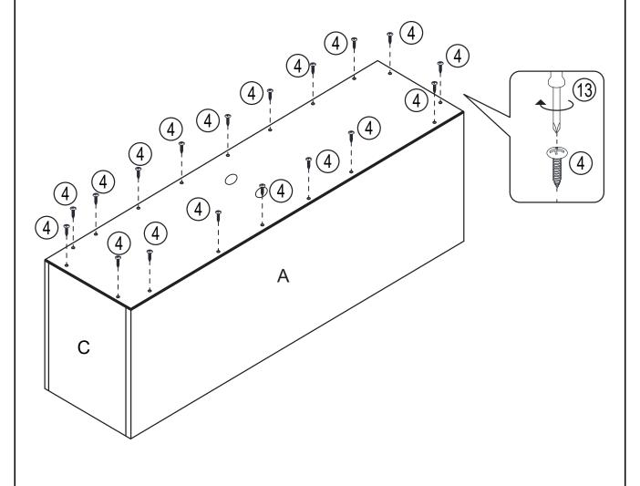
Attach Back Panel(H) to the Left Side Panel(C), Right Side Panel(F), Bottom Panel(B) and Top Panel(A) using Screw(4) with Screwdriver(13) as shown.
