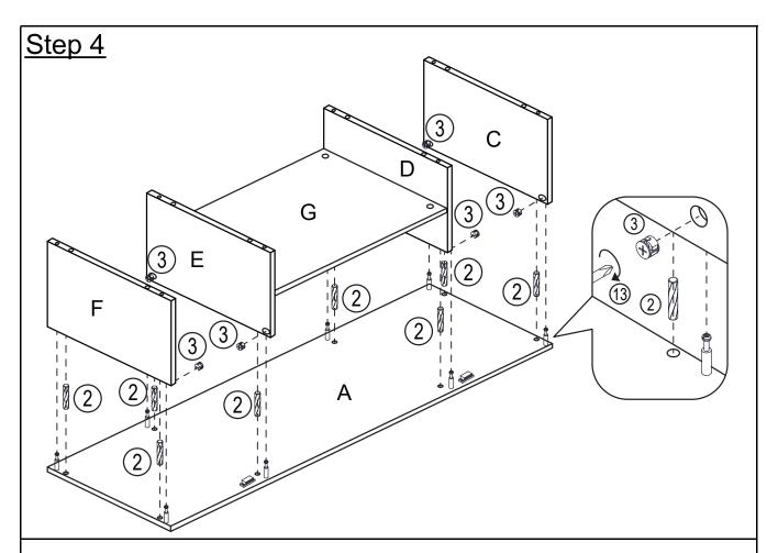
Attach Left Side Panel(C), Middle Left Side Panel(D), Middle Right Side Panel(E) and Right Side Panel(F) to the Top Panel(A) with Dowel(②), then insert Cam Nut(③) into Left Side Panel(C), Middle Left Side Panel(D), Middle Right Side Panel(E) and Right Side Panel(F) using Screwdriver(③) as shown.
