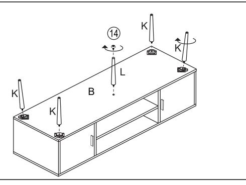
Attach Leg(K) and Support Leg(L) to the Bottom Panel(B), and then turn all legs clockwise to fasten them tightly.
