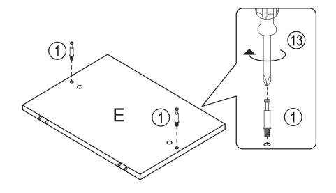
Insert Cam Bolt(1) into the mounting positions on Middle Left Side Panel(D) and Middle Right Side Panel(E) using Screwdriver(13) as shown.
