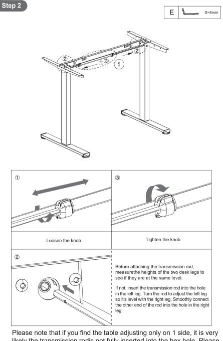
Please note that if you find the table adjusting only on 1 side, it is very likely the transmission rodis not fully inserted into the hex hole. Please revisit step 2 and insert the rod securely.
