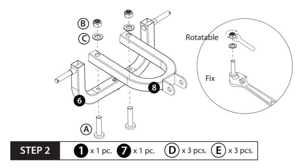
Fix the structure from Step 1 to Part 1 via Parts D (1 pc.) and E (1pc). Fix Part 7 to Part 1 via Parts D (2 pcs.) and E (2 pcs.).
